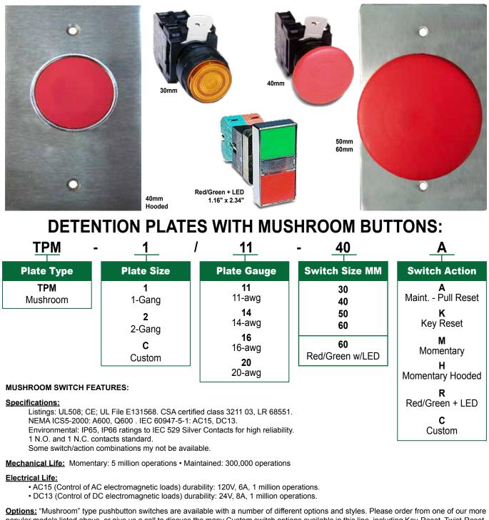
popular models listed above, or give us a call to discuss the many Custom switch options available in this line, including Key-Reset, Twist-Reset, Illuminated-any color, protective bezels and shrouds, additional N.O. or N.C. Switch Contacts, rotary switches and other options.
