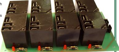
Eight control switch inputs are provided. Eight form C relay outputs are provided. A red status LED is provided for each relay.
