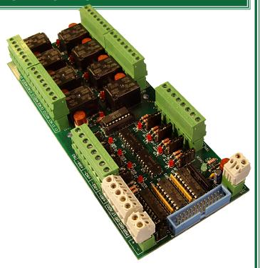
Field wiring connects to Phoenix type compression screw terminal plugs sized for 22 to 12 AWG stranded conductors. Control panel wiring is connected via a 26-pin male header. The mating female ribbon plug is provided.
